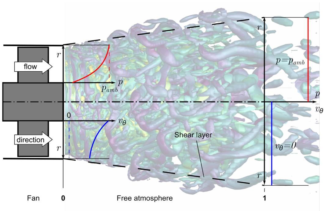
**Figure 2:** Schematic illustration of the static pressure recovery in the discharge of rotor-only axial fans. From location 0 immediately downstream of the trailing edge of the fan to location 1 far downstream the average static pressure must increase to ambient pressure.
