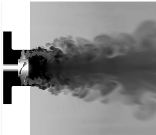
**Figure 1:** Meridional slice of a DES simulation of a low pressure axial fan with the instantaneous density distribution as contour, where brighter areas indicate higher values.
