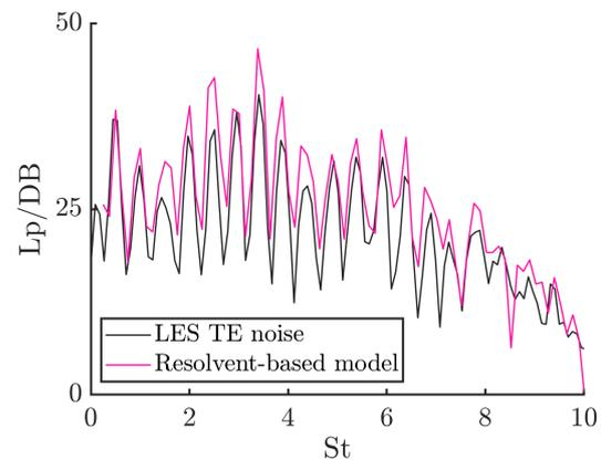
**Figure 3:** Comparison of the acoustic spectrum sampled near the trailing edge from the LES dataset and from the low-order model based on the leading resolvent mode of the flow.
