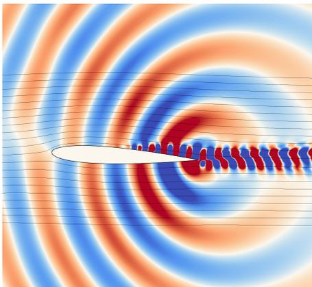
**Figure 2:** Pressure fluctuations from the leading SPOD mode of the flow around a NACA0012 airfoil at  $Re = 50\,000$ , revealing the coherent structures of the turbulent flow.
