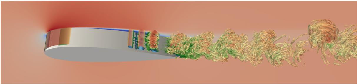
**Figure 1:** Snapshot of the turbulent structures ( $Q$ -criterion) developing around a NACA0012 airfoil at  $Re = 50\,000$  without tripping of the boundary layer. The streamwise velocity contours are given in the background.
