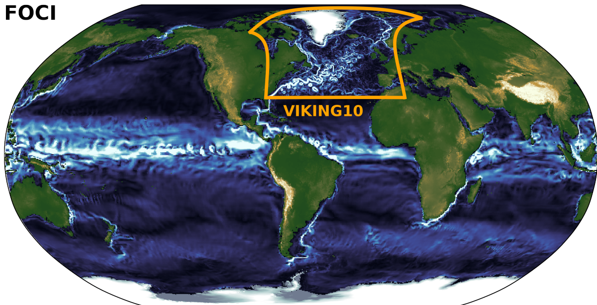
Figure 2: Snapshot of upper ocean current speed in a global coupled climate model simulation with FOCI-VIKING10. The default global ocean at 1/2° grid resolution clearly lacks mesoscale ocean features. By implementing the 1/10° North Atlantic nest VIKING10 an eddy-rich ocean is simulated in the refinement region (orange outline). Note, color scale highlights current speeds exceeding 0.5 m/s in white.
