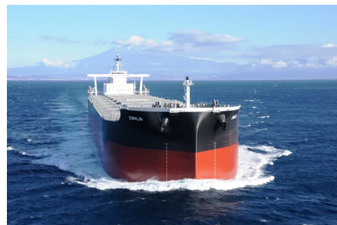
Figure 1: Example of sharp bow shape on a bulk carrier (courtesy of Japan Marine United Corporation)
