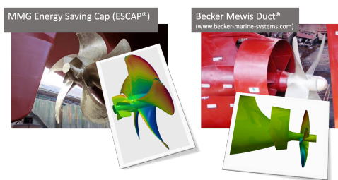
Figure 1: Examples of Energy-saving-devices (courtesy of MMG and Becker Marine Systems)
